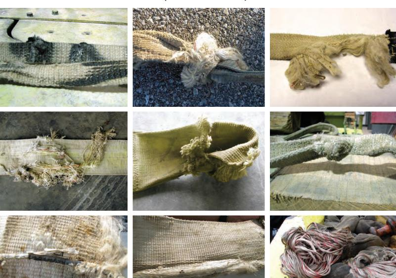
It doesn't matter whether it's a rope, strap, cable, chain, or hook. You should only store a device if it is in good operating condition. If your strap is cut, its strength capacity is less than its rated capacity. If your recovery chain has stressed links from the recent pull, then that's where it will break the next time it is put under stress. If your rope is frayed because it was laying on a sharp edge, you have compromised its ability to carry the load it was rated for when new.
