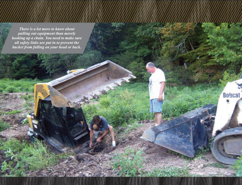
Before you try to extract any stuck vehicle with a cable, rope, or chain, consider the 28 tips described below. Remember, your goal is to have the pulling force exceed the immovable force — only then will the truck or stuck equipment move forward. If there is not enough force pulling forward, then whatever is stuck will not move.
