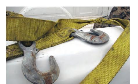
Knots significantly reduce the strength of any strap or tow rope. Straps are designed to be used flat. Knots reduce the strength of the web when it is bunched together and twisted into a tight knot. All of the tension is placed on less area.
