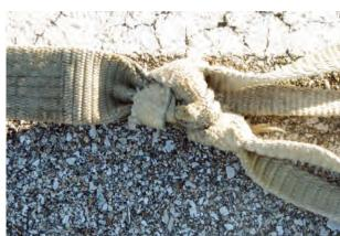
Tying two or more recovery straps together with a knot reduces the overall towing power. The rope is at full strength when it is flat and the fiber is not pinched together. The strength of the strap is now based on the strength of the knot.
