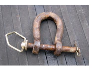
Using a regular hitch pin in lieu of what came with the clevis is a mistake.
