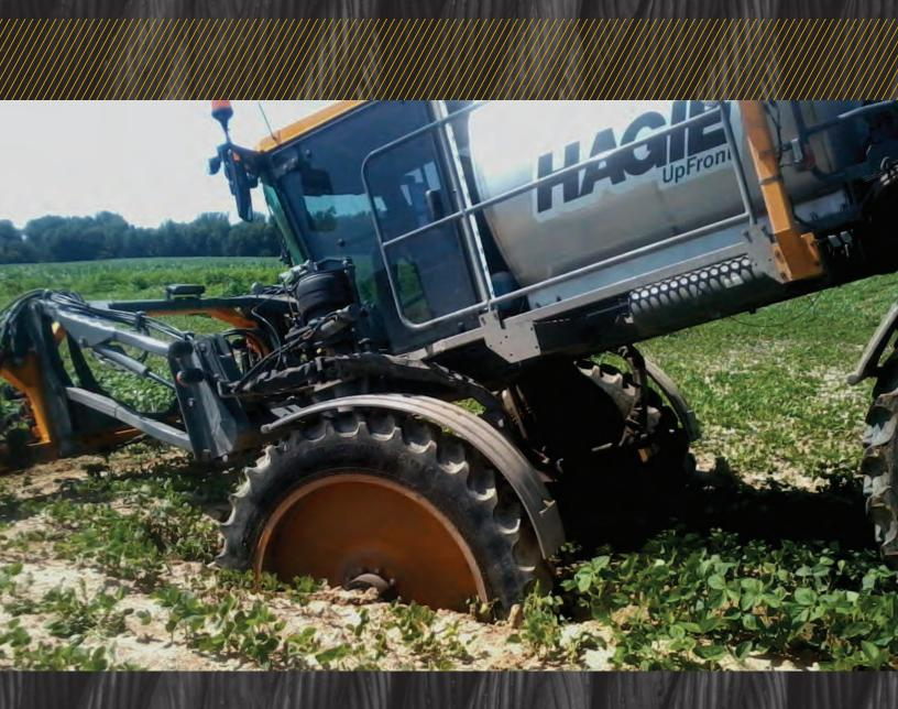
It takes more pulling strength to move something mired in the ground than it takes to pull the same object over the road. When you tow something on the road all you have to do is get the weight of the towed vehicle moving forward.
