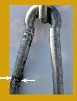
While commonly used on chains, these connectors cannot stand the stress they will encounter during vehicle or equipment extraction.
