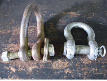
Never replace the original pin that came with your device with bolts from your bins or local hardware stores (left). If you need to replace the pin, replace it with a pin that is comparable to the pin that came with the original equipment at the time of purchase.
