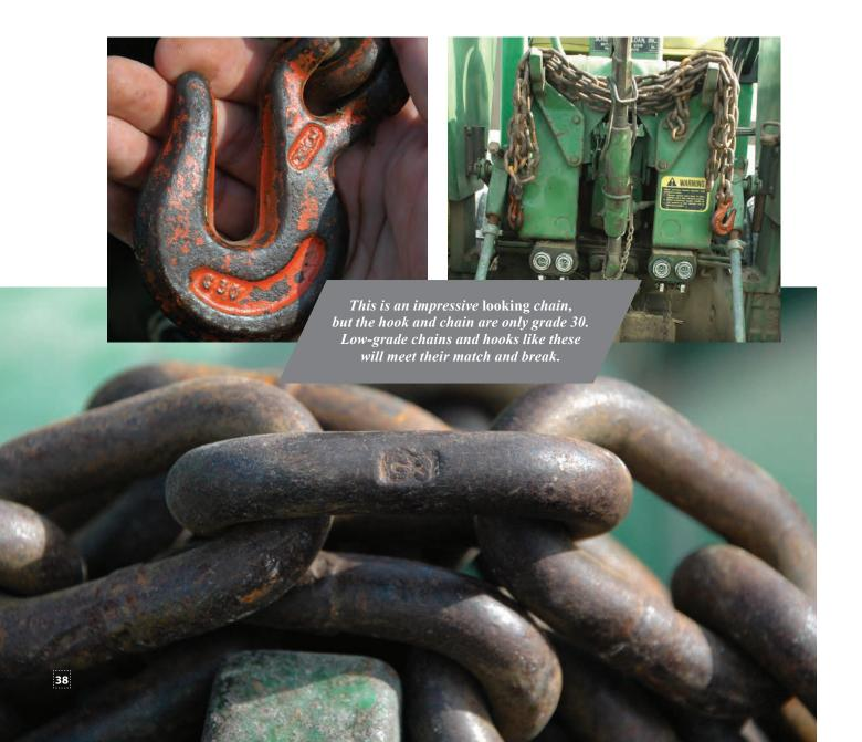
All this is not to say that chains will not work. For example, using chains from the shop might be good for pulling out light vehicles that are not deeply stuck in mud or those vehicles that can't get enough traction on ice or snow to move forward. And as long as you don't jerk them, you can use chains to extract heavier equipment as long as the chains are designed and rated for towing the weights they will encounter.
