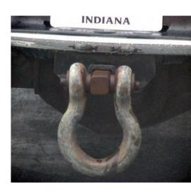
This equipment looks impressive, but looks can be deceiving. Always look for the ratings associated with each piece of equipment. In this case, pay particular attention to the receiver hitch platform and make sure it is rated equal to or greater than the pickup.
