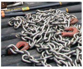
Never assume that a strong chain is enough. Always determine the strength of the hooks. The breaking point is the lowest number of the two.
