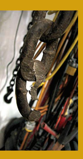
Chains are important for any farm or business. However, unless the chains have been inspected for faulty links, they will have limited use for extracting stuck equipment. Notice one of the links that was dragged on the ground and one with a broken link. Never put damaged chains back in service.
