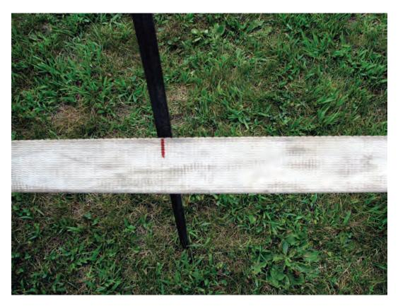
(Top) A red mark was made on the strap before extraction. This recovery strap stretched 8 inches during the extraction (below).
