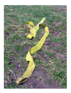
Should the clevis be rated more than the rope or the strap? Many think that you want the rope to fail before the clevis. A rope failure is a lot better than a chain, cable, hook, or clevis flying through the air. You want the weakest link to be the rope or strap.
