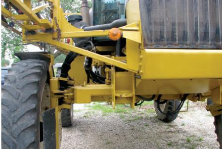
As a last resort, attaching to the truck hitch might be your only option. Understand that in most cases, manufacturers warn against using the hitch and attachment this way. Any damage will likely be the responsibility of the person or company doing the towing.
