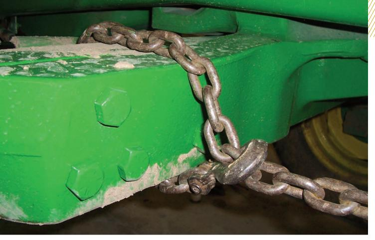
Grab hooks are designed to slide over the full link. Don't hook the tip of the grab hook into the opening of the link pulling on the tip of the hook. Pulling on the tip of the hook compromises the design capabilities of the grab hook.
