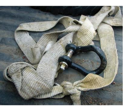
This clevis is solid, but all its strength is defeated by knotting up the strap.
