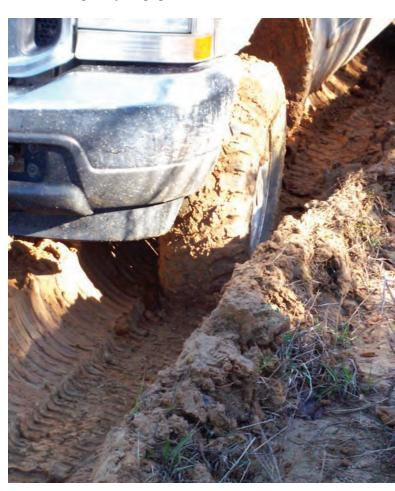
Ideally, you want to position the towing vehicle on higher ground. This will give you a mechanical advantage to overcome and negate the forces that hold the stuck equipment in the mud. It is easier on the towing vehicle if it can pull the stuck vehicle's wheels up and out of the hole and onto solid ground. If the towing vehicle is pulling forward or downward, it is forcing the stuck equipment into the immovable ground.
