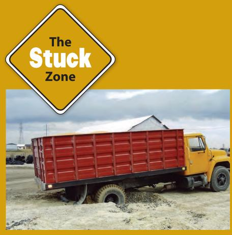
Since this truck is loaded with corn, the total weight that needs to be pulled out will be a lot more than the truck alone.
