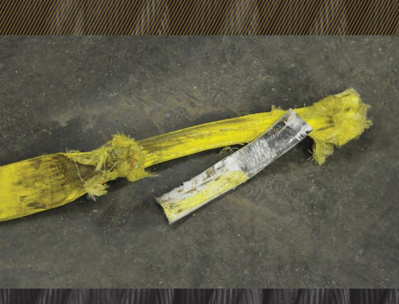
Straps and ropes used for recovery are made to withstand different stress levels based on how they are manufactured. The manufacturer includes a label on each device that provides users with valuable information and confirms what the manufacturer is willing to guarantee.
