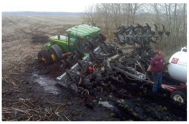
You need to be especially careful in a situation like this. Inspect all hoses and fittings after the tractor and wagon are pulled out to make sure no anhydrous has leaked. And before you try to make any extraction consider whether the wagon should be separated from the tractor, the wagon should be pulled out backward, and the anhydrous ammonia tank valves have been shut off.
