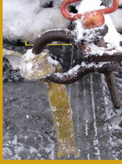
After this strap was torn, the operator tied a knot around the clevis and continued to pull equipment.
