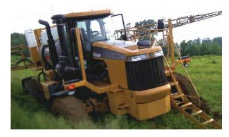
Before you extract this equipment, ask yourself some questions. What is in the tank? Can I drop the clean rinsing water to lighten the load? Could I transfer the spray solution safely to lighten the load?
