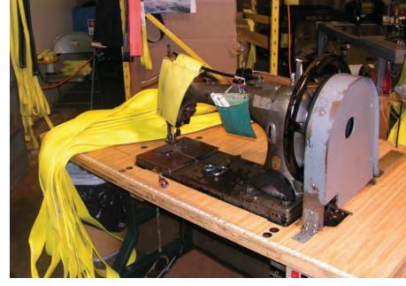
Strap manufacturers can repair damaged straps.
