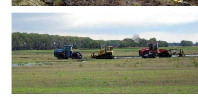
There should never be another person in the danger zone when you are extracting a stuck vehicle. The person on the four-wheeler is in great danger because a piece of metal or strap could come lose during the pulling process.
