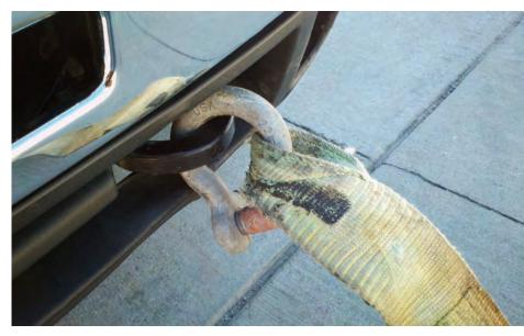
An improper strap attachment can pull apart the clevis.
