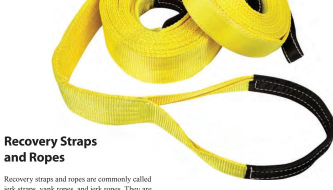
Recovery straps and ropes are commonly called jerk straps, yank ropes, and jerk ropes. They are designed and fabricated much differently than their counterparts used for towing. They are lighter than chains and cables. And unlike tow ropes and straps, recovery straps and ropes don't have any hardware attached to them and the material allows for stretching under tension.
