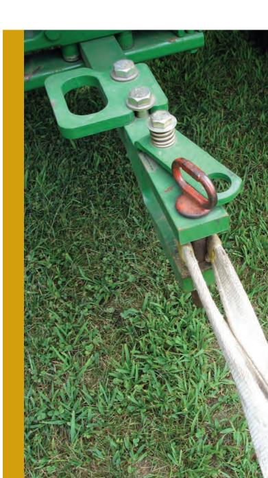
It is usually not a good idea to use a truck hitch to extract stuck equipment. In fact, many manufacturers' hitch tag instructions caution against using the hitch to pull out equipment.
