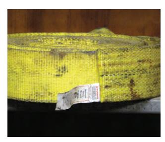
Keep this recovery strap in a container to protect it against damage from grease and sunlight.
