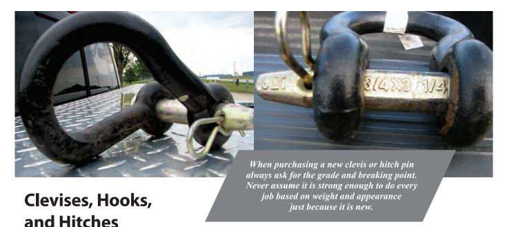
While most of the attention is devoted to straps, chains, ropes, and cables, it's important to realize the other items used to extract stuck vehicles also have ratings that are just as important. Remember that metal, if placed under enough stress, will break. And when it does, it could lead to severe injuries, or worse, death.
