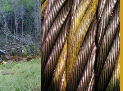
You also have to pay attention to how many of the wires are cut — if enough get cut, the integrity of the cable will be compromised. Each cut or broken strand reduces the cable's overall strength.
