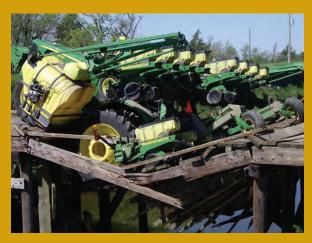
Always take a close look at the integrity of the fuel, hydraulics, dye, herbicide-treated seed, and coolant systems before you make any decision to move the equipment.
