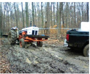
It will be rather difficult to extract this truck because the towing tractor does not have firm ground to work on. Also, the attachment point being used on the tractor is not the drawbar. A homemade frame may not have the force required to extract the truck.
